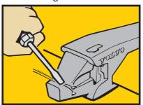
6 Thoroughly clean the adapter's nose and the hole for the lock pin, so that the tooth and lock pin can be fitted in the
