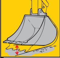
3 To make tooth mounting easier, angle back the bucket a bit so that the adapters face slightly upwards.
